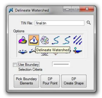
b) Click the Pick Boundary Elements button and select the element representing the tin hull (the boundary of the TIN file) as shown in the screenshot below. Data Point to accept.
